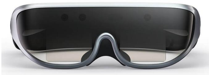
Voler worked with Rokid to create the entire electronics design. We integrated multiple sensor technologies—HD Camera, Time-of-flight camera (3D), audio (play and record), and included WiFi and Bluetooth connectivity. There is an HD video display projected on the lens in front of your eye. Given the multiple use cases planned—from mission critical tasks to hands-free operations, the battery life was critical and we were able to deliver a custom board that just sipped power.
